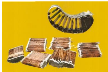
Fig 25 A/C Cooler under repair
