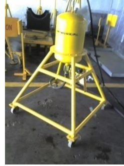
Figure 4 DORNIER AIRCRAFT COMPRESSOR WASHING RIG
