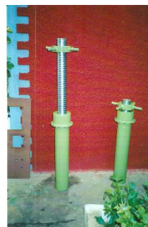
FIGURE 10 TEN TON HYDRAULIC CYLINDER WITH LOCKS
